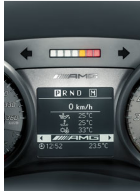
AMG instrument cluster with 7-LED upshift indicator.
