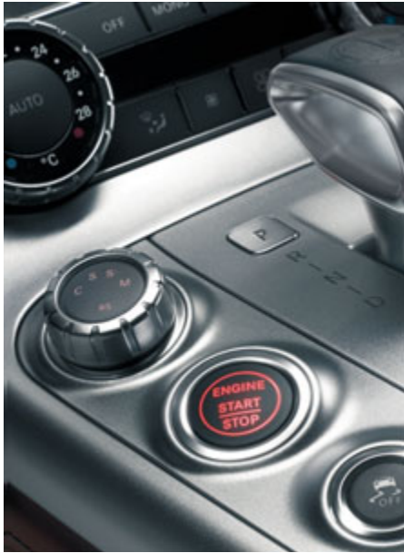
The AMG DRIVE UNIT with E-SELECT selector lever and KEYLESS-GO start function.
