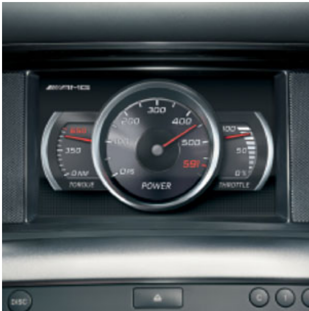
Optional extra. AMG Performance Media, torque, output and accelerator position display.
