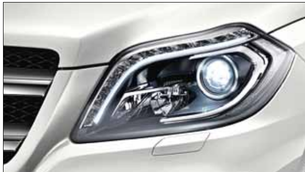
Adaptive Highbeam Assist automatically always provides the best possible headlamp range, thereby improving visibility for the driver.
