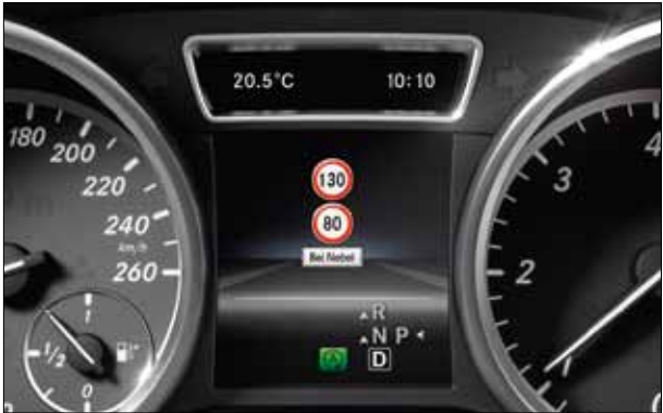
Speed Limit Assist can also display temporary speed limits in the instrument cluster.
