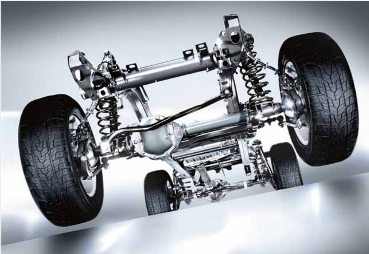
Rigid axles are extremely resilient, even when subjected to heavy loads during off-road driving, and offer constant ground clearance as well as optimum traction.
